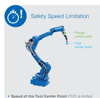
and monitored. If no TCP is defined, the Flange Center Point (FCP) is limited and monitored
