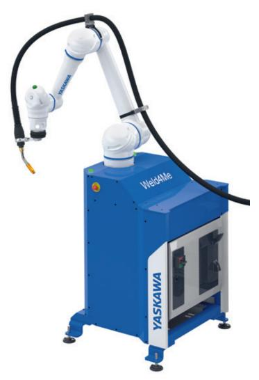
As an alternative or supplement to manual MIG/MAG welding with air-cooled welding equipment, the Weld4Me robot station offers all the advantages needed. It has a small footprint and is easy to move with a hand pallet truck, and it brings the consistent quality of robotic welding to your production processes.
